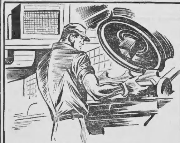
MANY INDUSTRIAL PRODUCTS ARE MADE IN AIR CONDITIONED ROOMS SO THAT OUTSIDE TEMPERATURE CHANGES WILL NOT AFFECT THEIR DIMENSIONS WHILE THEY ARE BEING MANUFACTURED
